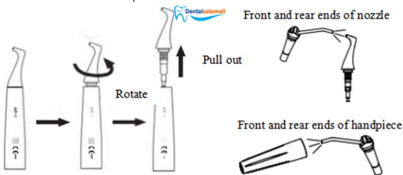
Fig. 7 handpiece cleaning diagram
