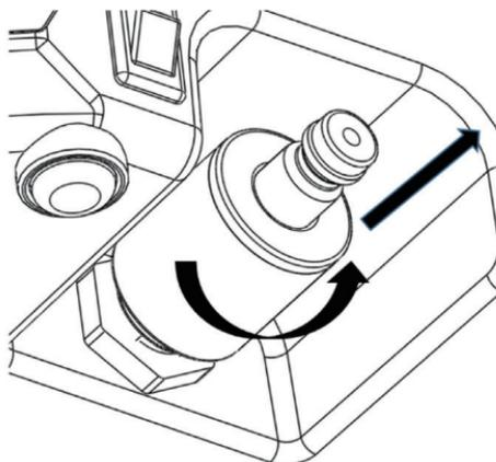
Fig. 8 Schematic diagram of filter replacement
