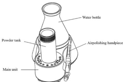
Fig. 1 Front view of main unit
